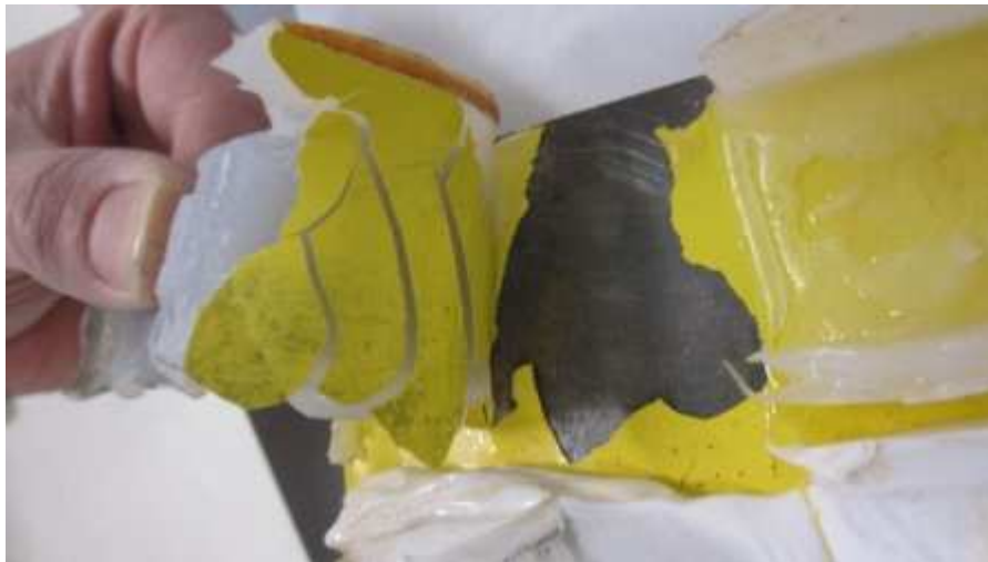
Picture 1. Yellow coating pulled from the steel. Adhesion to the coating 100%
