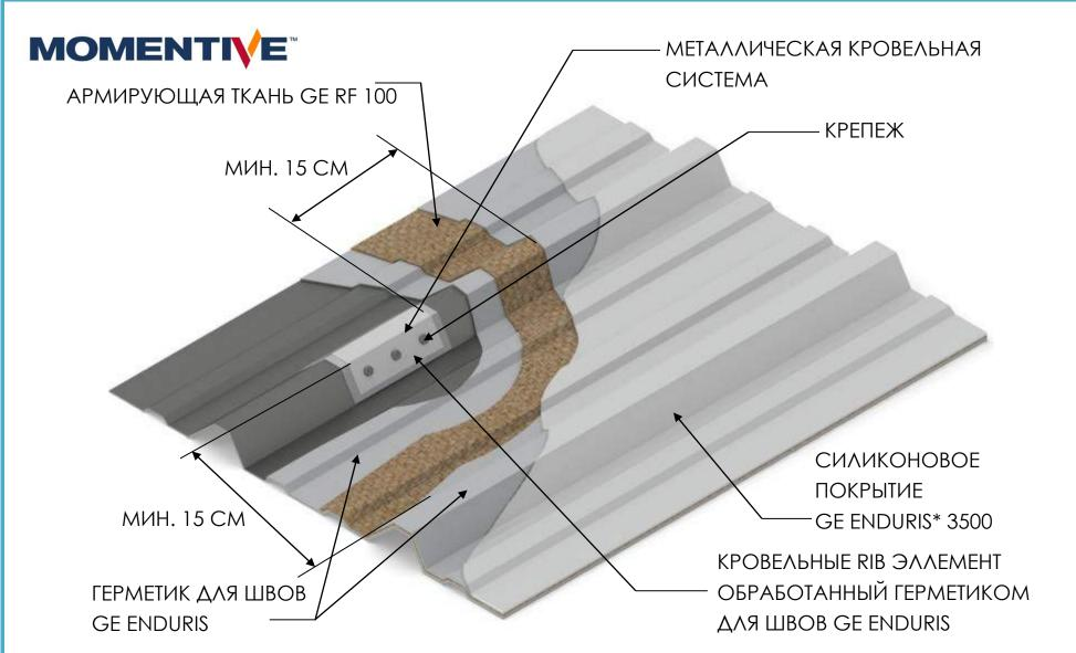
NOTE: RIB CAPS ARE REQUIRED OVER BROKEN RIBS; AFTER INSTALLATION, SEAL THE RIB CAP PERIMETER AND FASTENERS WITH ENDURIS SEAM SEALANT
