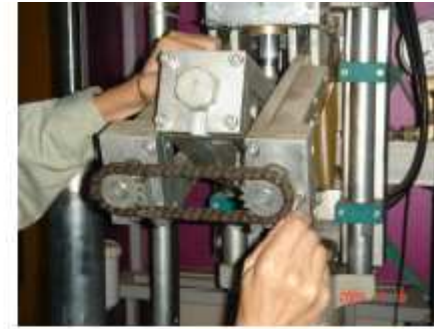
Loose 10 screws at bottom side of scale (not need to take away screws).
