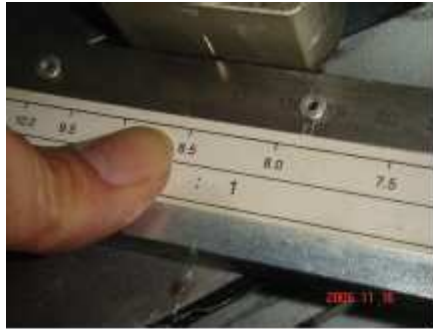
Original scale Mixing ratio by volume is 8.3:1 (11.4:1 by weight), need to fix @ 8.7:1 (12:1 by weight)
