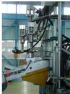
Adjust scale bolt by spanner, Try to restore suck pipe at vertical position.
