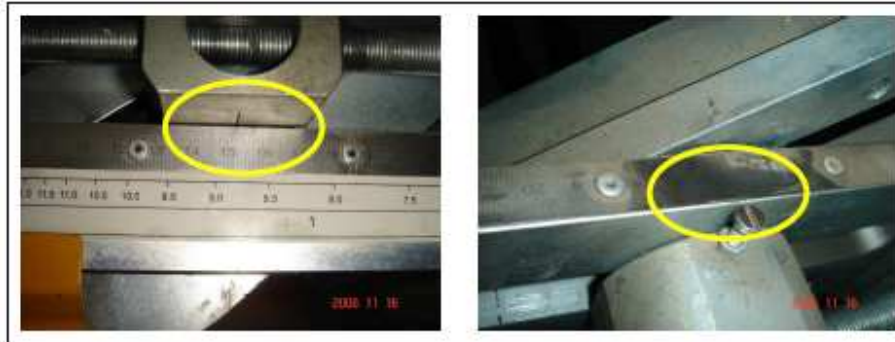
After adjusting, scale is same as that on suck pipe.
