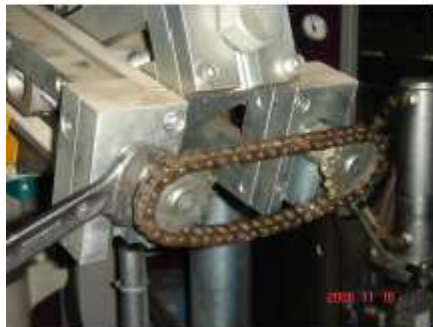
Adjust screw bolt of scale with a suitable spanner, move scale from 8.4 to 8.7.
